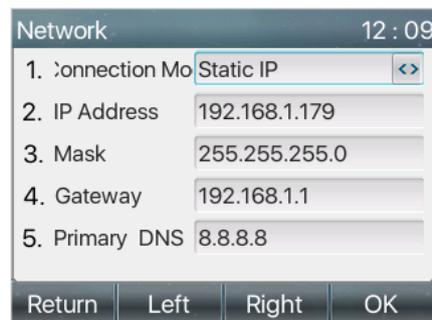
**Picture 112 - Static IP network mode**
