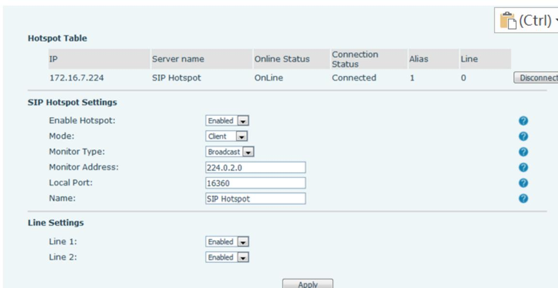
**Picture 82 - SIP hotspot client configuration**
