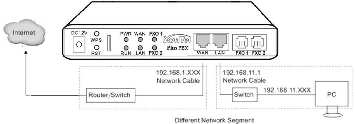
Note: The IP address of LAN port of the PBX and the IP address of PC must be at the same network segment, while that of WAN port is at a different network segment.
