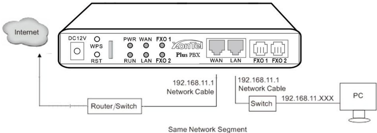
Note: The IP address of PC and that of WAN port of the XonTel Plus PBX are at the same network segment.
