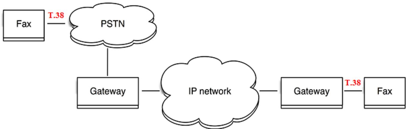
**Pass-through:** Under the pass-through mode, fax signal is not converted and fax traffic is carried in RTP packets. It uses the G.711 A or G711U codec in order to reduce the damage to fax signal.
